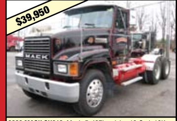
$39,950 2002 MACK CH613. Mack @ 427hp, Jake, 13-Spd, 12K F/A, 44K R/A, Camelback Susp, 3-Line Wet Kit, Double Frame, 242k Miles, Stk# A9019
